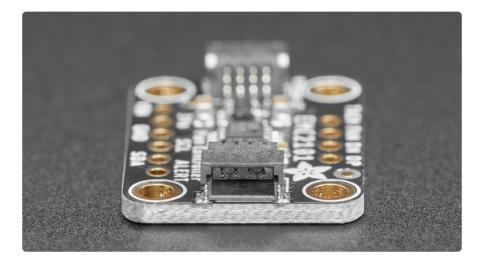
Delivered to you on our custom Stemma QT form factor PCB, the Adafruit EMC2101 breakout is ready to help you integrate a fan into your project by making it easy to use with a range of devices. A voltage regulator and 5V tolerant pins allow you to use it with 3.3V or 5V microcontrollers or single board computers. The included included SparkFun qwiic (https://adafru.it/Fpw) compatible STEMMA
