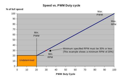
This can vary from fan to fan. Ideally, this information will be given in a fan's datasheet. For example, this if from the datasheet for a Delta Electronics AUB0912VH fan:
