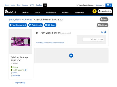
To view the data that has been logged from the sensor, click on the graph next to the sensor name.
