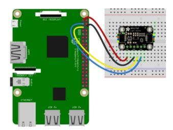
Pi 3V to sensor VCC (red wire)
