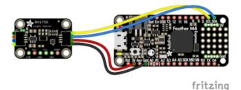
Board 3V to sensor VIN (red wire)
