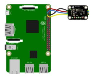
Pi 3V to sensor VCC (red wire)
