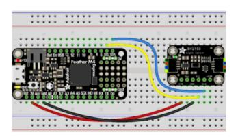
Board 3V to sensor VIN (red wire)
