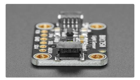
To make things easier and a bit more flexible, we've also included <u>SparkFun Qwiic</u> (htt ps://adafru.it/Fpw) compatible <u>STEMMA QT</u> (https://adafru.it/Ft4) connectors for the I2C bus so you don't even need to solder!
