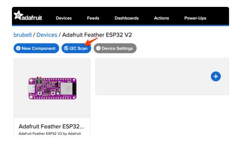
You should see the BH1750's default I2C address of 0x23 pop-up in the I2C scan list. If the jumper on the underside of the board is soldered, this address will be changed to 0x5c.
