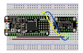
Board 3V to sensor VIN (red wire)
