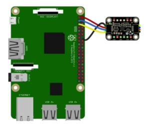
Pi 3V to sensor VCC (red wire)
