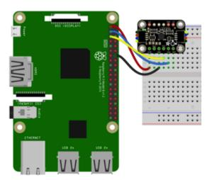
Pi 3V to sensor VCC (red wire)
