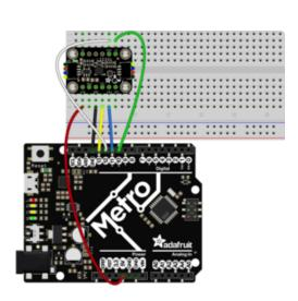
Connect **Vin** to the power supply, 3V or 5V is fine. Use the same voltage that the microcontroller logic is based off of Connect **GND** to common power/data around
