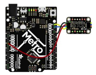
Connect **board VIN** (**red wire**) to **Arduino 5V** if you are running a **5V** board Arduino (Uno, etc.). If your board is **3V**, connect to that instead.
