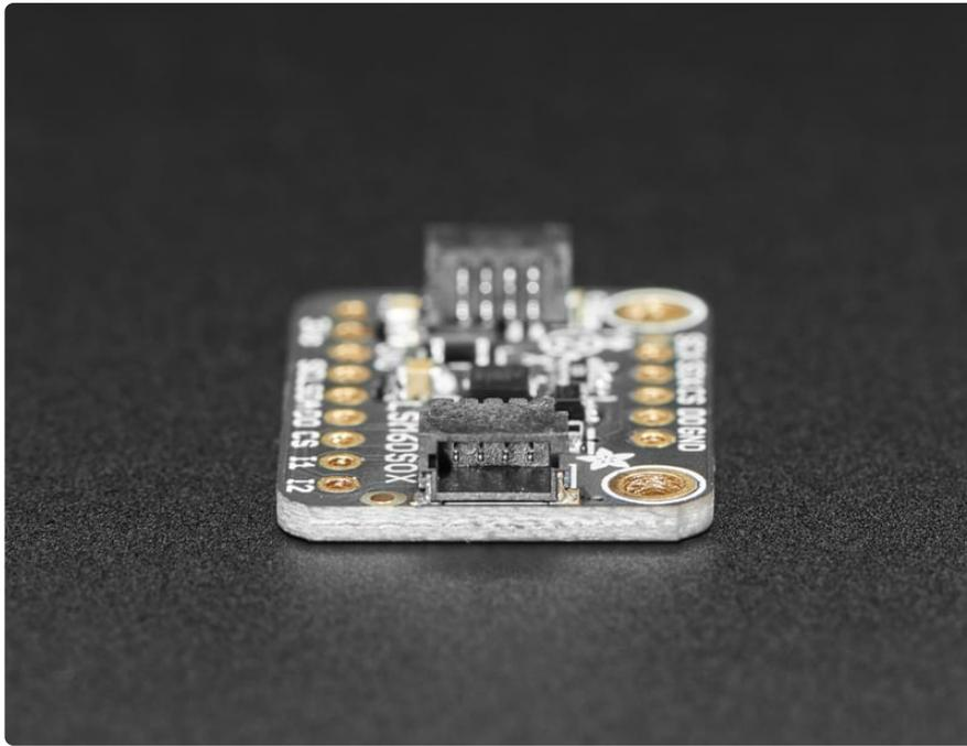
Additionally since it speaks I2C you can easily connect it up with two wires (plus power and ground!). We've even included [SparkFun qwiic \(https://adafru.it/Fpw\)](https://adafru.it/Fpw) compatible [STEMMA QT \(https://adafru.it/Ft4\)](https://adafru.it/Ft4) connectors for the I2C bus so **you don't even need to solder!** Just wire up to your favorite micro with a plug-and-play cable to get 6 DoF data ASAP.
