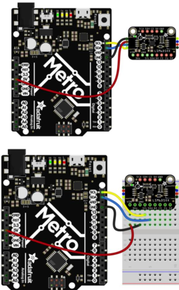
Connect board **VIN** (red wire) to Arduino **5V** if you are running a **5V** board Arduino (Uno, etc.). If your board is **3V**, connect to that instead.
