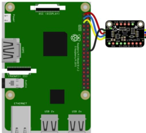
Pi 3V to sensor VCC (red wire)
