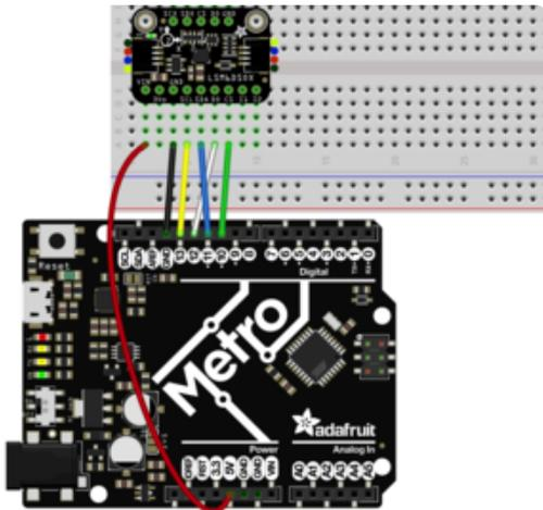
Connect **Vin** to the power supply, 3V or 5V is fine. Use the same voltage that the microcontroller logic is based off of
