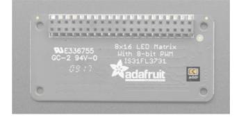
The default I2C address for the Bonnet is  $0 \times 74$ . Solder this jumper closed to change it to  $0 \times 70$  to avoid I2C address conflicts, if needed.
