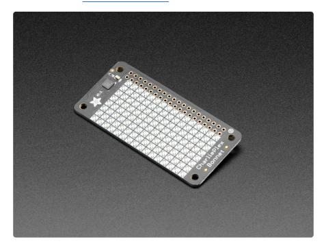
What is particularly nice about this Bonnet is the I2C LED driver chip has the ability to PWM each individual LED in a 16x8 grid so you can have beautiful LED lighting effects, without a lot of pin twiddling. Simply tell the chip which LED on the grid you want lit, and what brightness and it's all taken care of for you. You get 8-bit (256 level) dimming for each individual LED.
