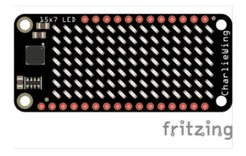
Assemble the CharlieWing by soldering headers onto the board. Once assembled, plug it into a Feather!
