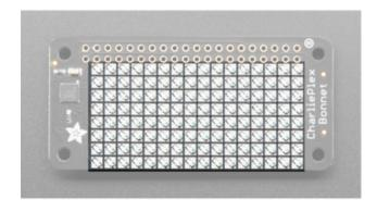
The 8 x 16 LED matrix on the CharliePlex Bonnet provides 128 LEDs.
