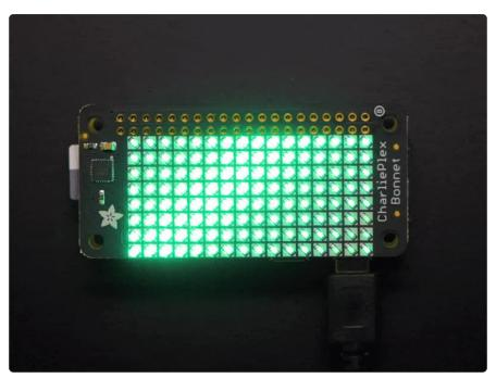
You won't be able to look away from the mesmerizing patterns created by this **Adafruit CharliePlex LED Matrix Display Bonnet**. This 16x8 LED display can be placed atop any Raspberry Pi computer with a 2x20 connector, for a beautiful, bright grid of 128 CharliePlexed LEDs. It even comes with a built-in CharliePlex driver that is run over I2C.
