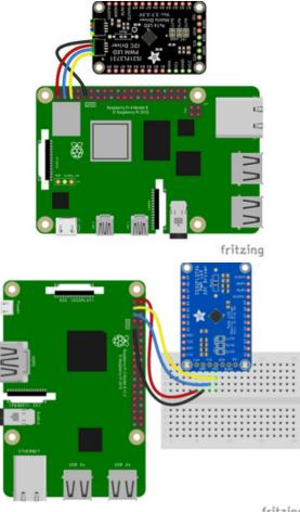
Pi 3V3 to breakout VIN Pi GND to breakout GND Pi SCL to breakout SCL Pi SDA to breakout SDA
