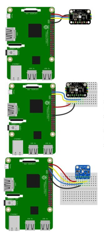
Pi 3V3 to sensor VIN (red wire on STEMMA QT version) Pi GND to sensor GND (black wire on STEMMA QT version) Pi SCL to sensor SCK (yellow wire on STEMMA QT version) Pi SDA to sensor SDI (blue wire on STEMMA QT version)
