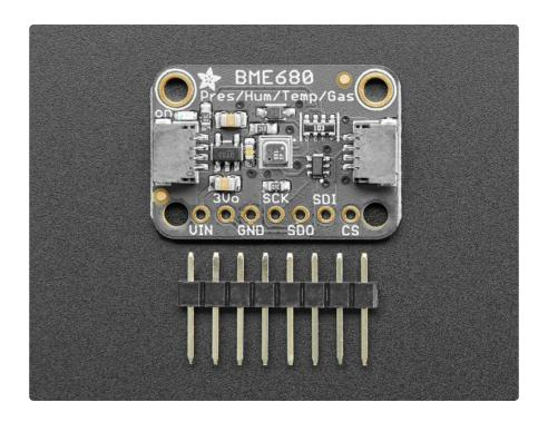
The BME680 takes those sensors to the next step in that it contains a small MOX sensor. The heated metal oxide changes resistance based on the volatile organic compounds (VOC) in the air, so it can be used to detect gasses & alcohols such as Ethanol, Alcohol and Carbon Monoxide and perform air quality measurements. Note it will give you one resistance value, with overall VOC content, it cannot differentiate gasses or alcohols.
