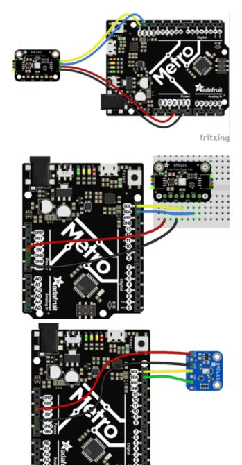
Connect Vin (red wire on STEMMA QT version) to the power supply, 3-5V is fine. Use the same voltage that the microcontroller logic is based off of. For most Arduinos, that is 5V. For 3.3V logic devices, use 3.3V
