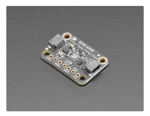
The long awaited BME680 from Bosch gives you all the environmental sensing you want in one small package. This little sensor contains **temperature**, **humidity**, **barometric pressure** and **VOC gas** sensing capabilities. All over SPI or I2C, at a great price!
