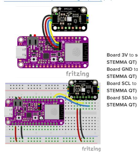
Board 3V to sensor VIN (red wire on STEMMA QT) Board GND to sensor GND (black wire on
