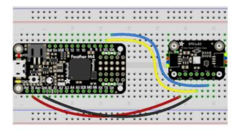
Board 3V to sensor VIN (red wire on STEMMA QT version) Board GND to sensor GND (black wire on STEMMA QT version) Board SCL to sensor SCK (yellow wire on STEMMA QT version) Board SDA to sensor SDI (blue wire on STEMMA QT version)
