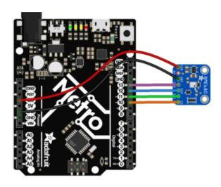
Connect **Vin** to the power supply, 3V or 5V is fine. Use the same voltage that the microcontroller logic is based off of Connect **GND** to common power/data ground
