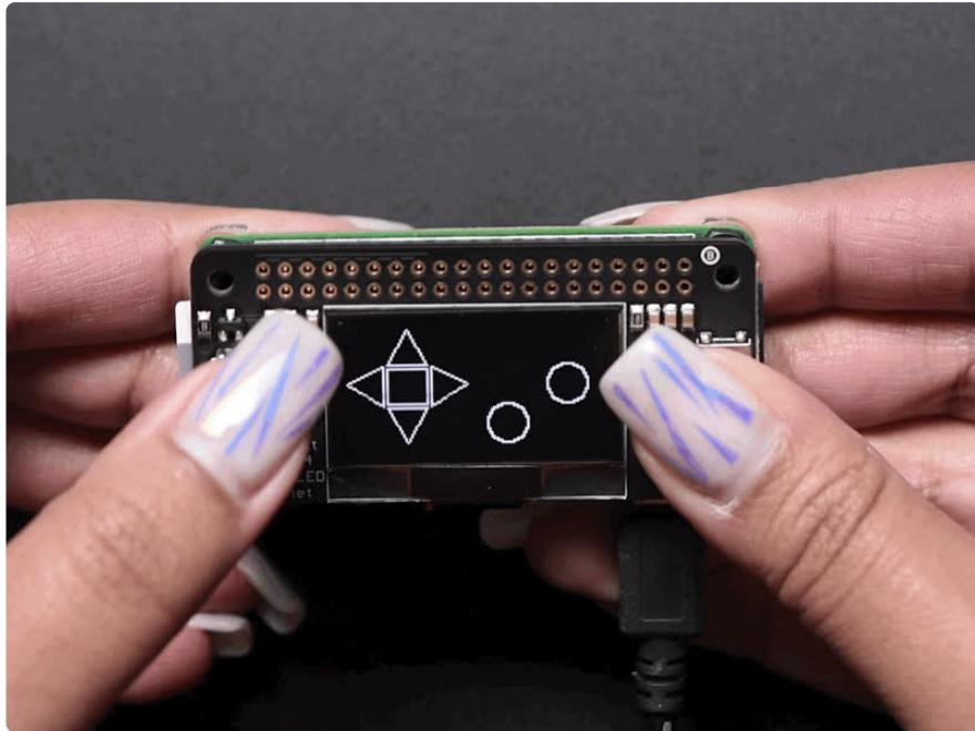
If you'd like a compact display, with buttons and a joystick - we've got what you're looking for. The Adafruit 128x64 OLED Bonnet for Raspberry Pi is [the big sister to our mini PiOLED add-on](#) (<http://adafru.it/3527>). This version has 128x64 pixels (instead of 128x32) and a much larger screen besides. With the OLED display in the center, we had some space on either side so we added a 5-way joystick and two pushbuttons. Great for when you want to have a control interface for your project.
