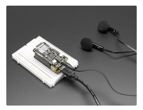
Bend all audio files to your will with the **Adafruit Music Maker FeatherWing!** It's a funsize version of our <u>Music Maker shield for Arduino</u> (http://adafru.it/1790)! This powerful shield features the VS1053, an encoding/decoding (codec) chip that can decode a wide variety of audio formats such as MP3, AAC, Ogg Vorbis, WMA, MIDI, FLAC, WAV (PCM and ADPCM). You can do all sorts of stuff with the audio as well such as adjusting bass, treble, and volume digitally.
