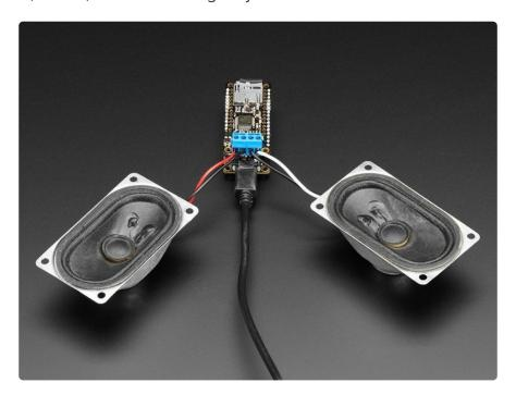
All this functionality is implemented in a light-weight SPI interface so that any Feather Board can play audio from an SD card. There's also a special MIDI mode that you can
