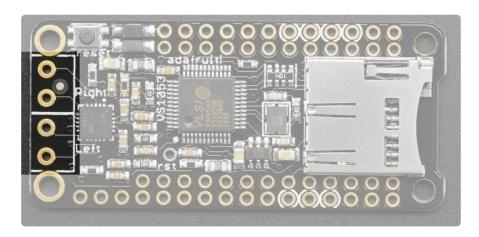
This is the bridge-tied-load output from the VS1053 through the amplifier chip. Connect to 4 to 8 ohm speakers. If you don't need both outputs, just keep one disconnected. Don't connect the outputs together! Nor can you connect the outputs to another amplifier - they are for direct connection to a speaker only!
