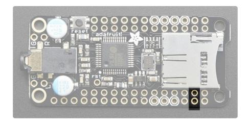
This is the UART data pin that is connected to the MIDI RX on the VS1053. If you short the jumper on the back to put it in MIDI mode, you can send data from the **TX** pin.
