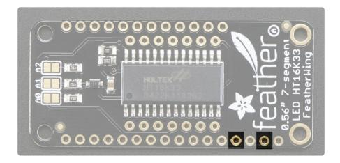
The LED matrix uses only the **3V** and **GND** pins for power and logic. Current draw depends on how many LEDs are lit but you can approximate it as about 40mA for most uses. Check the PCB file/schematic to verify which pin is ground!
