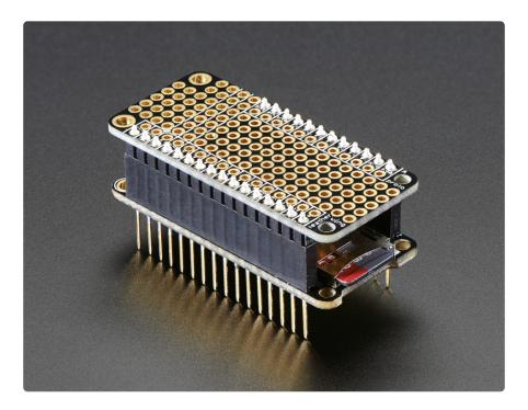
First is the **FeatherWing Proto** - a prototyping add-on for all Feather boards. Using our <u>Feather Stacking Headers</u> (http://adafru.it/2830) or <u>Feather Female Headers</u> (http://adafru.it/2886) you can connect a FeatherWing on top or bottom of your Feather board.
