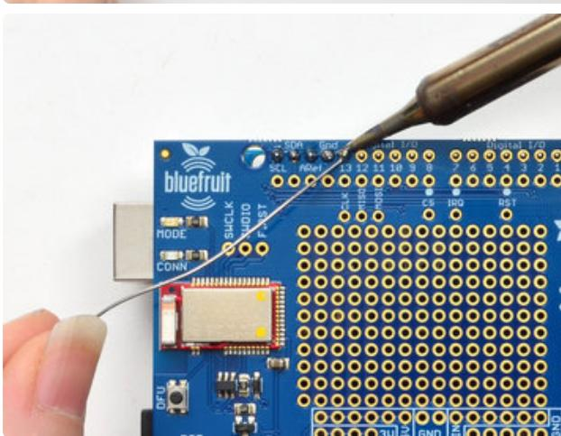
Solder in all the header on the top strips
