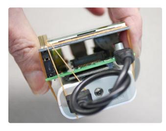
The package could be slimmed down considerably; there's a huge amount of empty space between the PiTFT and Raspberry Pi (even more with a Model A board). Advanced makers could squeeze a slim LiPo battery and a 5V boost converter in there, connecting to the expansion header at the right edge of the TFT board instead of the side-protruding USB power connector. The result would be similar in size to some consumer point-and-shoot digital cameras.
