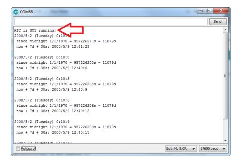
Whenever the RTC chip loses all power (including the backup battery) it will reset to an earlier date and report the time as 0:0:0 or similar. The DS1307 won't even count seconds (it's stopped). Whenever you set the time, this will kickstart the clock ticking.
