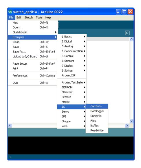
This sketch will not write any data to the card, just tell you if it managed to recognize it, and some information about it. This can be **very** useful when trying to figure out whether an SD card is supported. Before trying out a new card, please try out this sketch!
