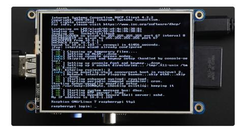
One fun thing you can do with the display is have it as your main console instead of the HDMI/TV output. Even though it is small, with a good font you can get 20 x 40 of text. For more details, check out <a href="https://github.com/notro/fbtft/wiki/Boot-console">https://github.com/notro/fbtft/wiki/Boot-console</a> (https://adafru.it/cXQ)
