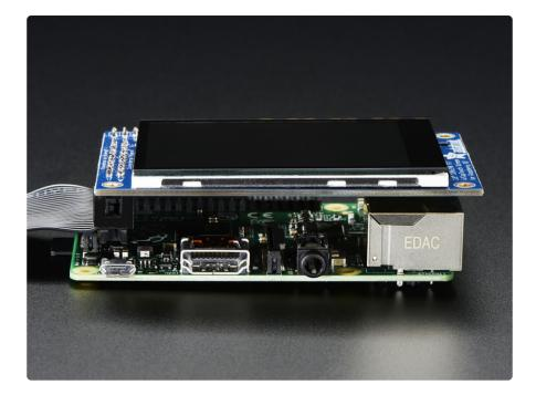
It's designed to fit nicely onto the Pi Model A or B rev 2 but also works perfectly fine with the Model B+ as long as you don't mind the PCB overhangs the USB ports by 5mm, see the photos above. Model B rev 1 have an older layout for the I2C pins and won't be able to use the touch screen
