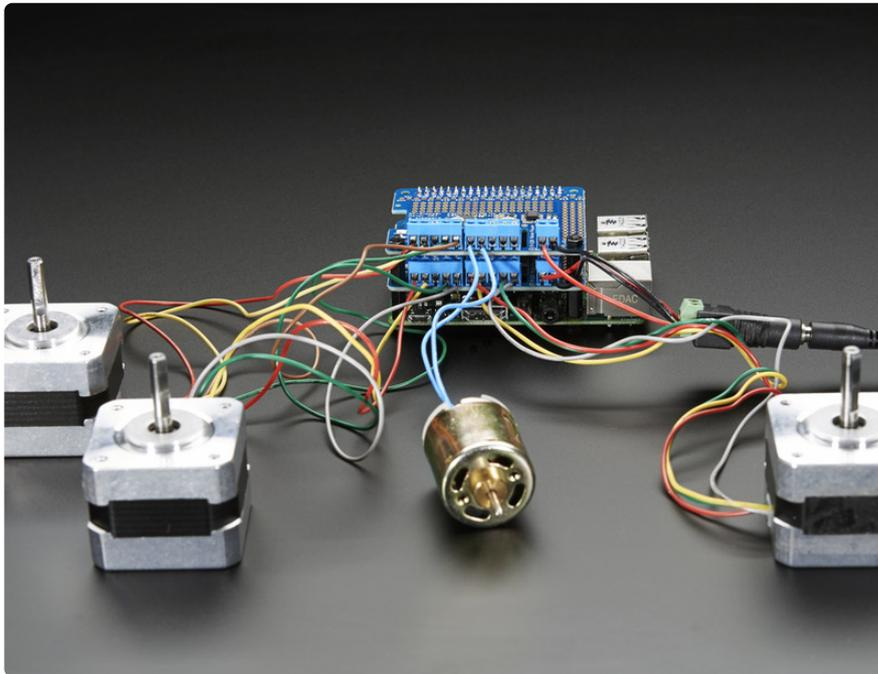
Motors are controlled TB6612 MOSFET driver: with **1.2A per channel current capability** (20ms long bursts of 3A peak), a big improvement over L293D drivers and there are built-in flyback diodes as well.
