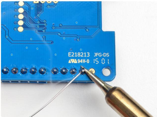
Flip over the board and solder in all of the terminal block pins
