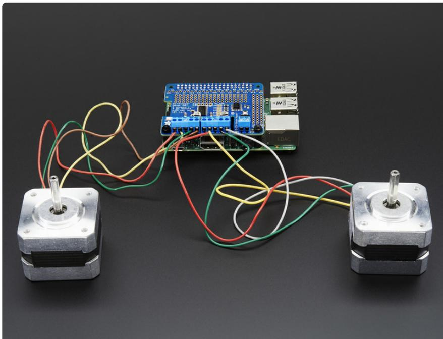
Since the Raspberry Pi does not have a lot of PWM pins, we use a **fully-dedicated PWM driver chip** onboard to both control motor direction and speed. This chip
