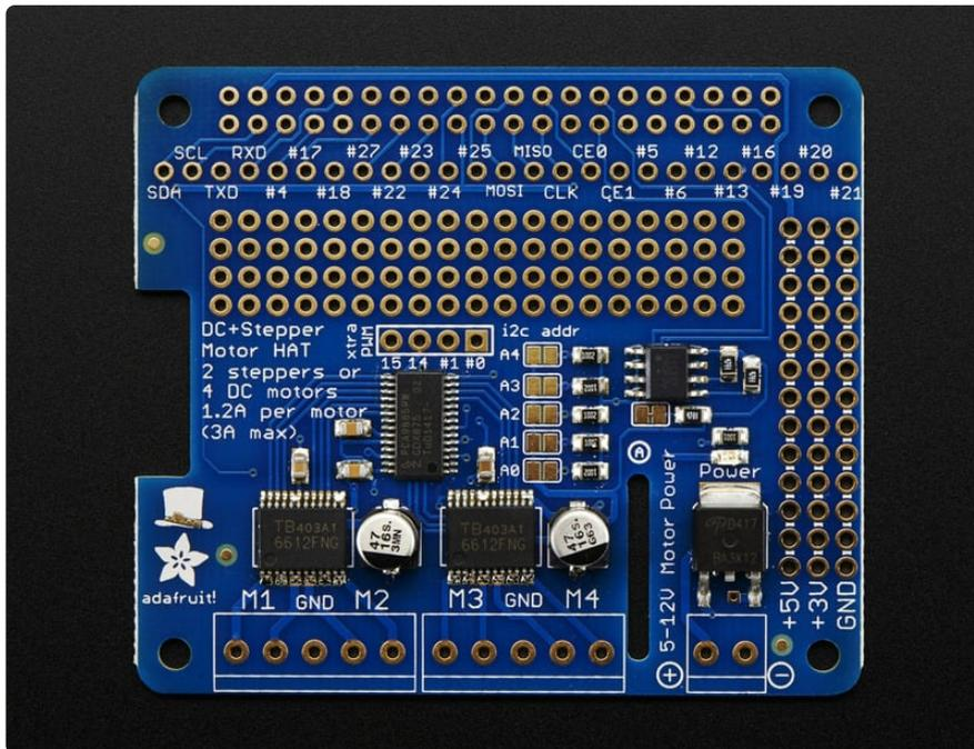
We even had a little space so we added a polarity protection FET on the power pins and a bit of prototyping area. And the HAT is assembled and tested here at Adafruit so all you have to do is solder on the included 2x20 plain header and the terminal blocks.
