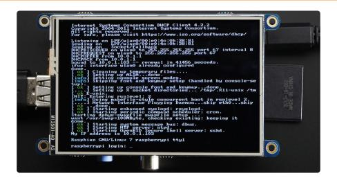
One fun thing you can do with the display is have it as your main console instead of the HDMI/TV output. Even though it is small, with a good font you can get 20 x 40 of text. For more details, check out <a href="https://github.com/notro/fbtft/wiki/Boot-console">https://github.com/notro/fbtft/wiki/Boot-console</a> (https://adafru.it/cXQ)
