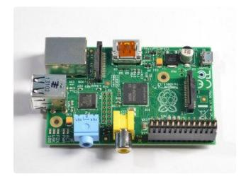
Plug the extra tall female header into the GPIO port on the Pi as shown. Make sure its seated nice and flat
