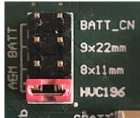
Fig. 2 - Jumper AEM_BATT set to 196 HVC ENYCAP™ (by default populated as 4.2 V / 4 F)
