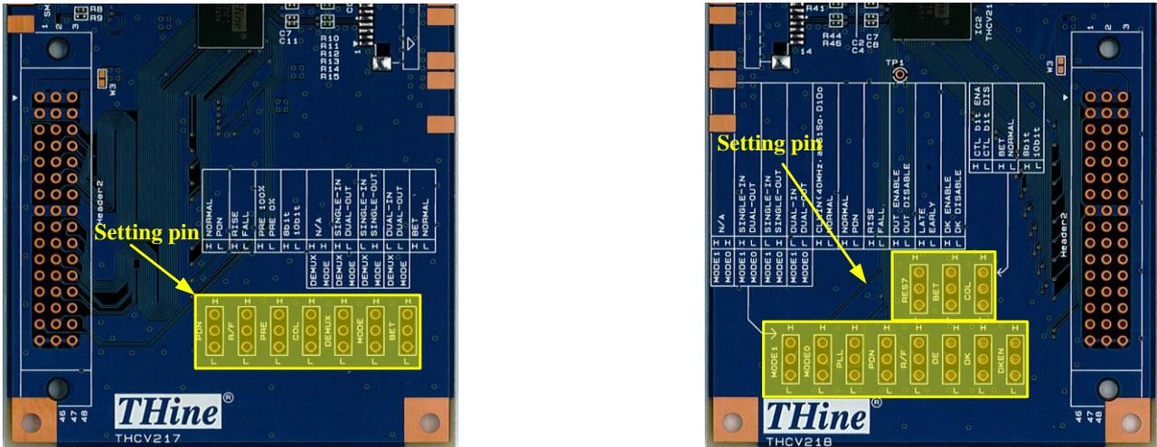
Figure 8 Position of Function Setting Pin
