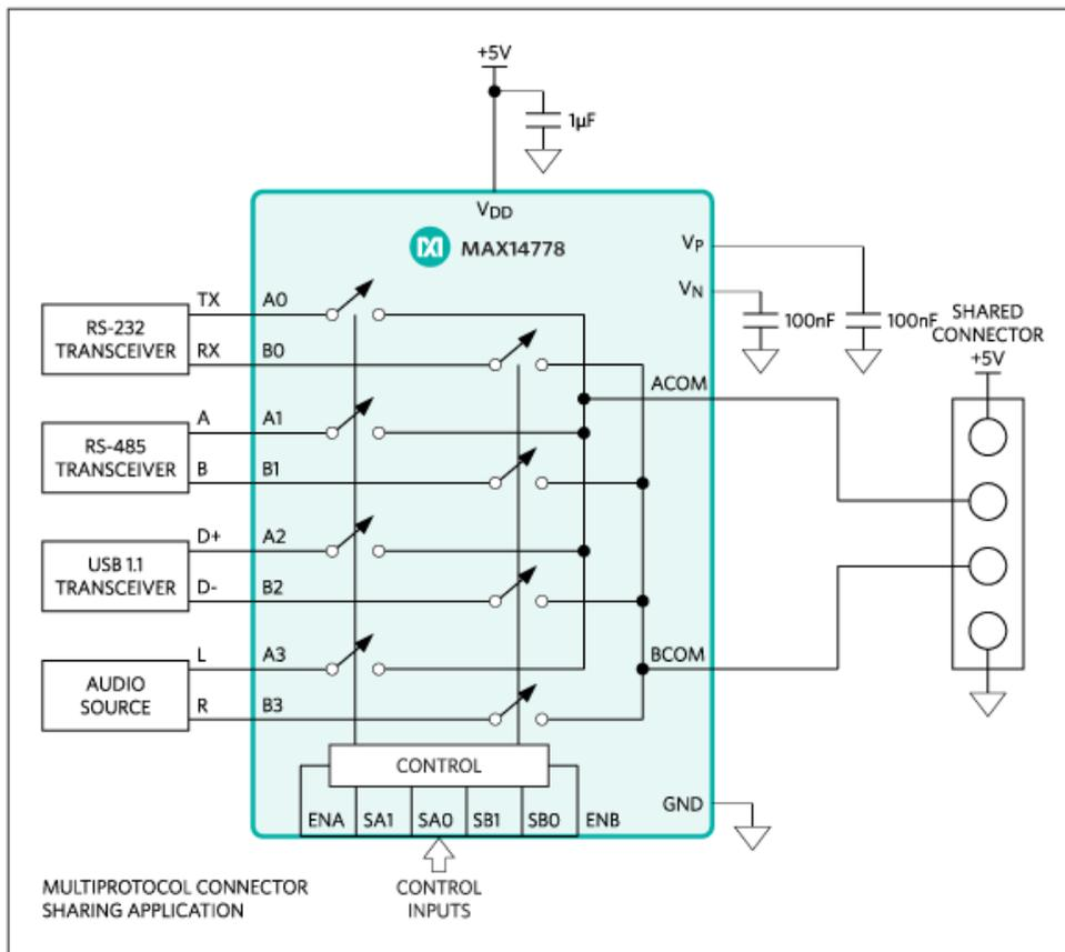
Figure 4. On-chip charge pumps allow the MAX14778 to implement multiprotocol sharing, amongst other functions, with signals as large as  $\pm 25V$  while operating on a single 3.0V to 5.5V supply.
