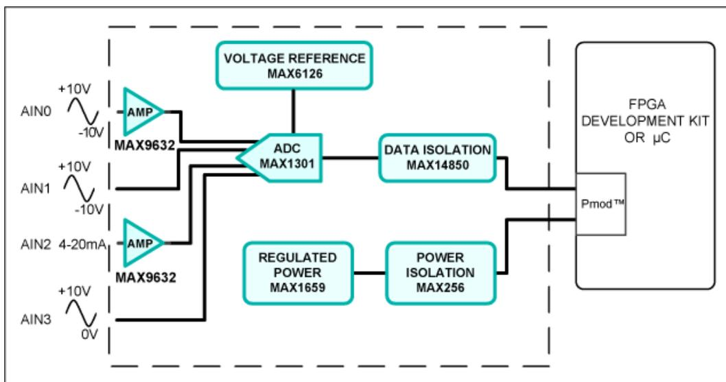
Figure 2. The Santa Fe reference design (top) implements a four-channel AFE with 16-bit resolution and on-board galvanic isolation as shown in the block diagram (bottom).
