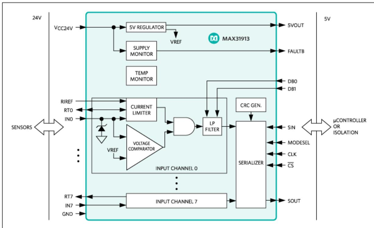
Figure 3. A MAX31913 industrial, octal, digital-input translator/serializer allows 24V signals from sensors and switches to interface directly with low-level CMOS logic.
