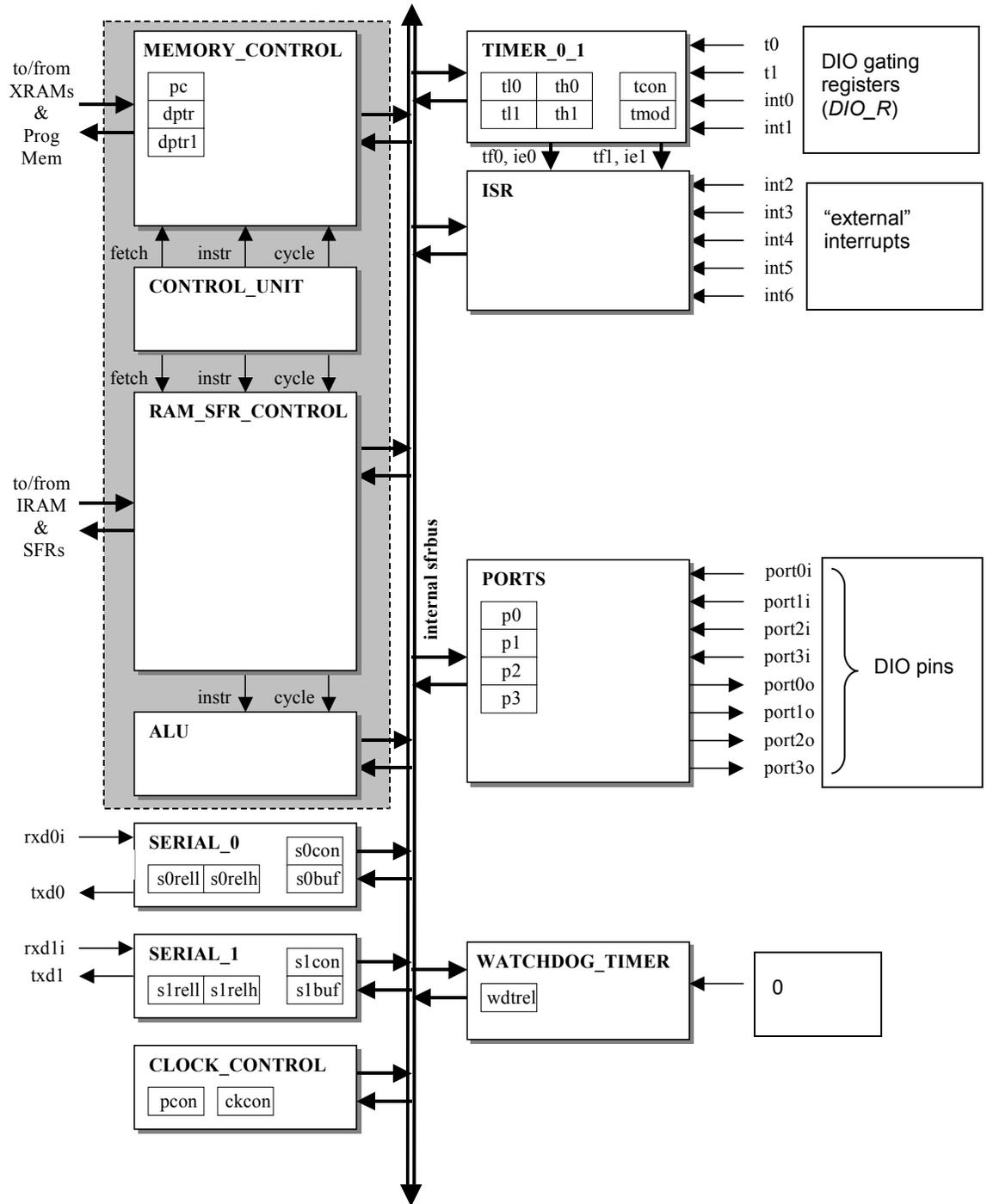
Figure 6-2: 80515 MPU Block Diagram
