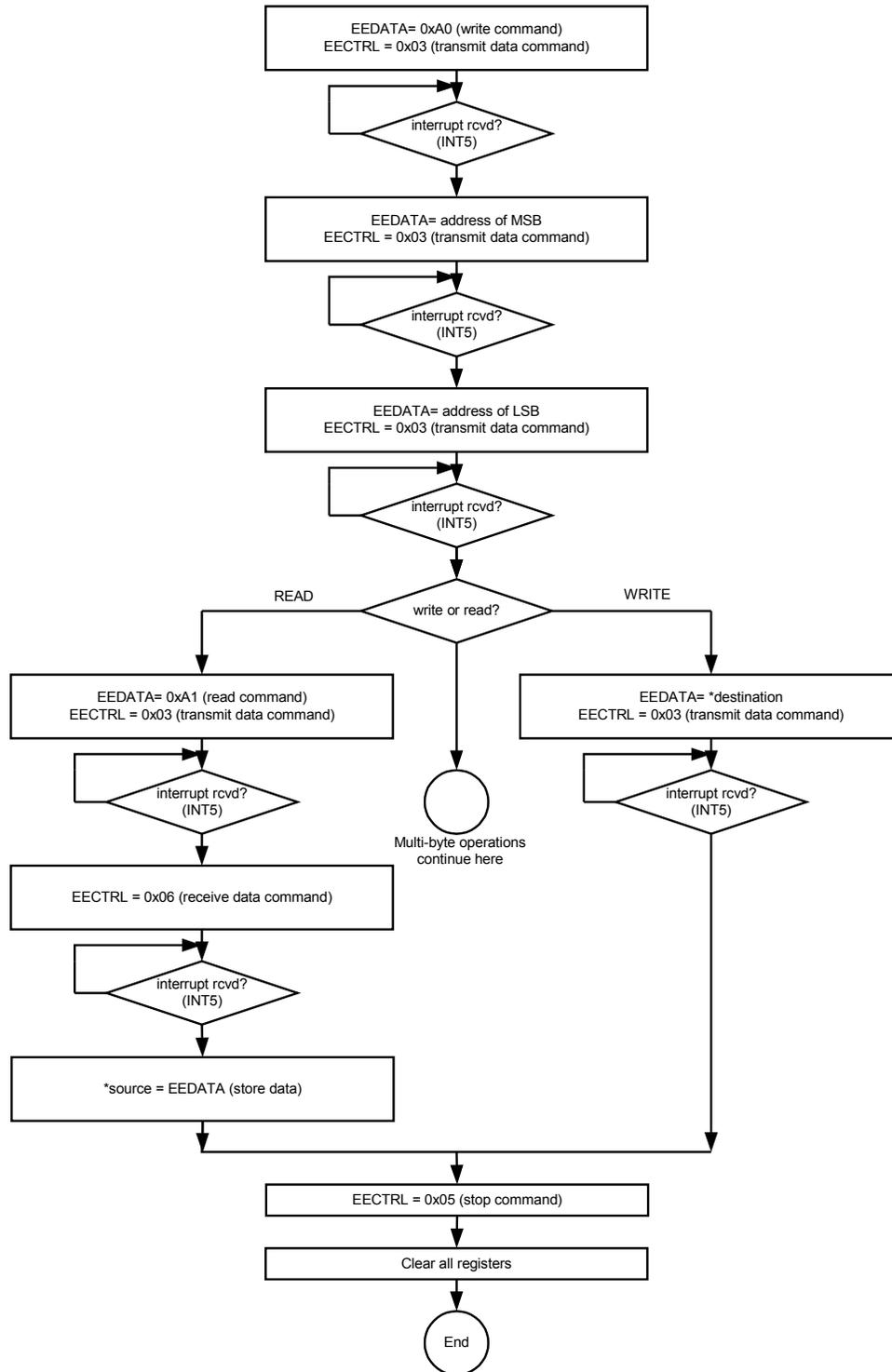
Figure 5-19: Single-Byte Read/Write
