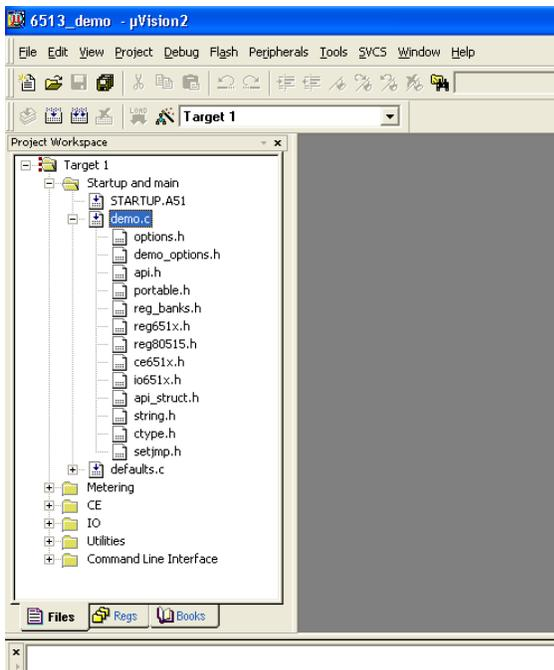
The Project Workspace screen on the left side of the window shows the main components of the source (Startup and main, Metering, CE, IO, Utilities, Command Line Interface) in folders. Folders can be opened by clicking on the plus sign next to them. Opening the folders will display the source files associated with them. Opening the source files will display the header files used by them.
