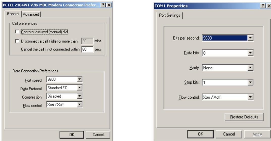
**Figure 3-1: Port Speed and Handshake Setup (left) and Port Configuration Setup (right)**
