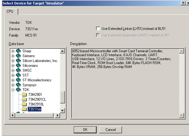
Under *Project* → *Options for Target1*, select the *Target* tab and enter the values in the fields as shown above. Confirm by clicking *OK*.
