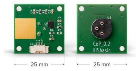
Driver circuit board for a quick evalution of HISbasic series IR emitters
