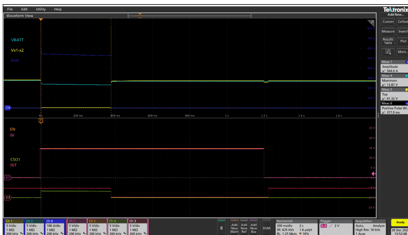
Figure 43 I-t wire protection test with circa 540 A scope depicting 200 ms/DIV
