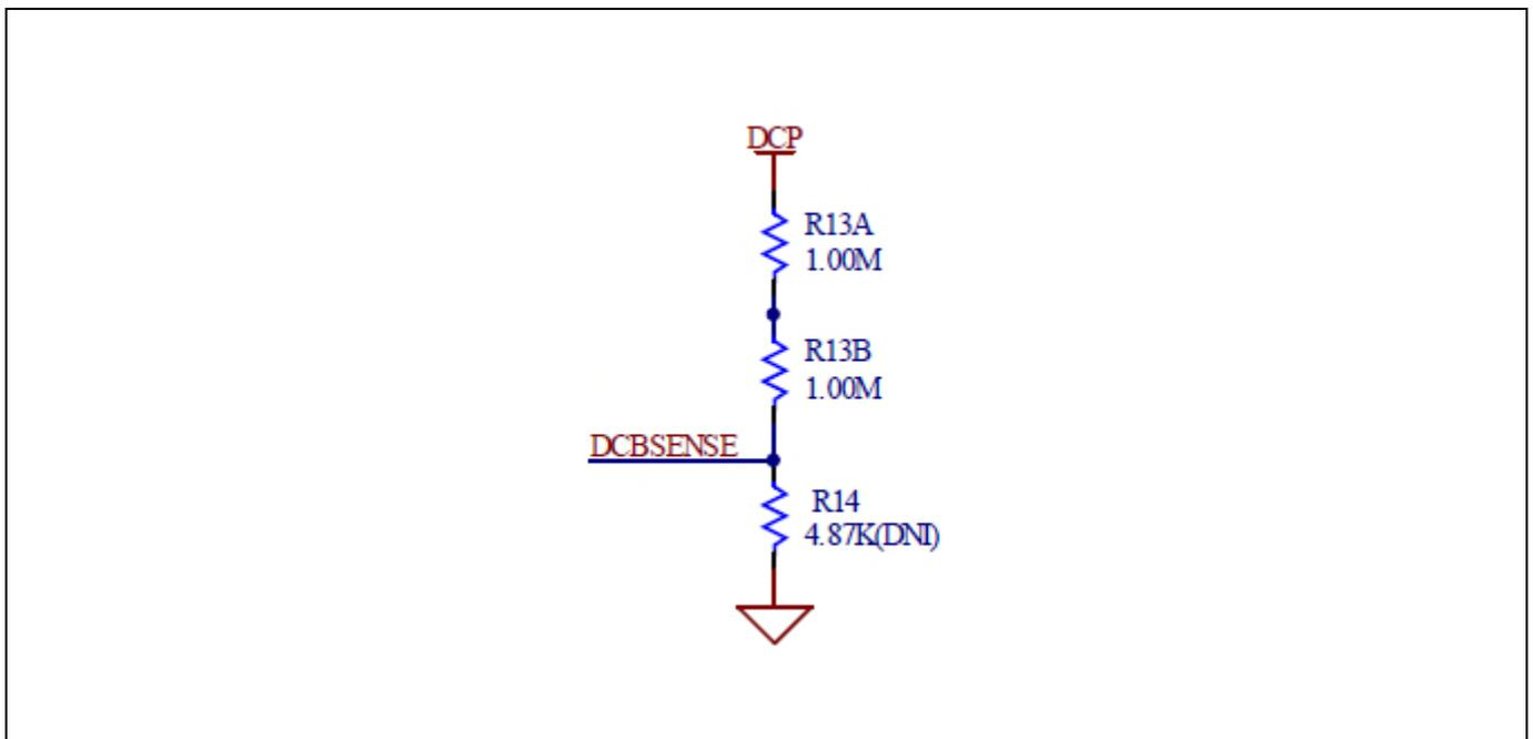
**Figure 11 DC bus sense resistor on EVAL-M1-05-84D evaluation board**
