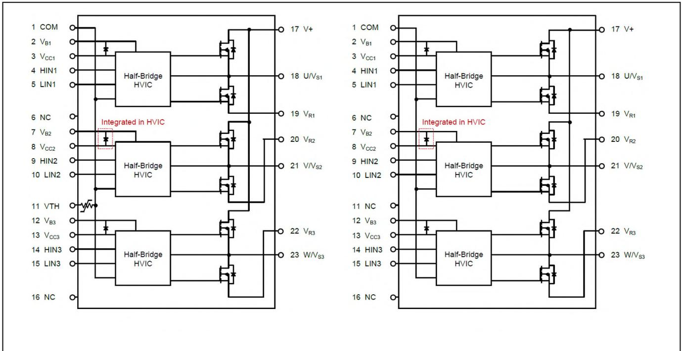
**Figure 2 CIPOS™ Micro internal electrical schematic**
