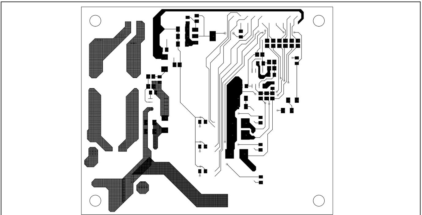
**Figure 19** Bottom layer routing of the EVAL-M1-05-84D
