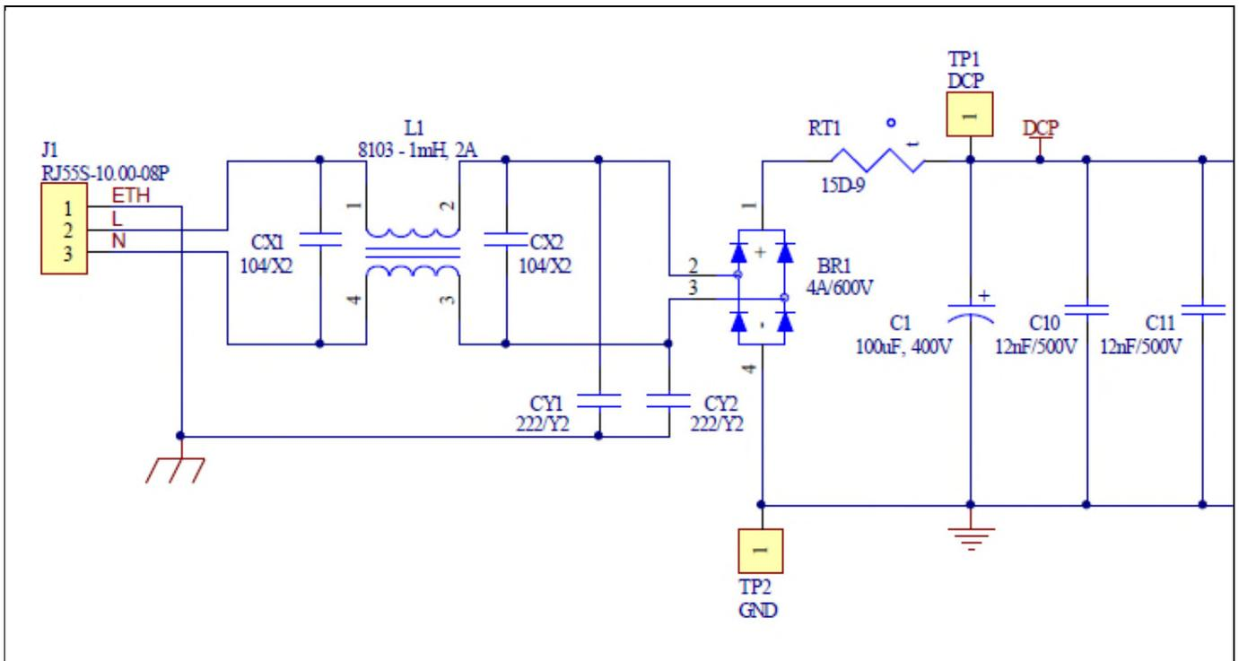
**Figure 12 Schematic for EMI input filter and AC/DC section of the EVAL-M1-05-84D evaluation board**
