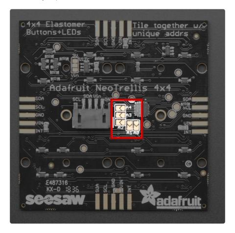
Each one of these is used to hard-code in the address. If a jumper is shorted with solder, that sets the address.
