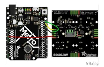
Wiring is easy, solder the four **VIN GND SDA SCL** pads to wires and then connect to your Arduino compatible:
