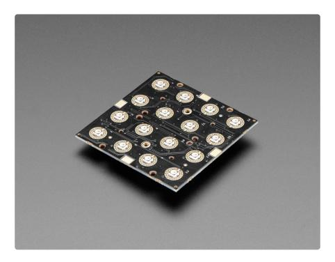
These 4x4 button pad boards are fully tile-able and communicate over I2C. With 5 address pins, you've got the ability to connect up to 32 together in any arrangement you like. With our trusty seesaw I2C-to-anything chip (https://adafru.it/Cmk), you don't even need to manage the NeoPixel driving. That's right! Both the button management
