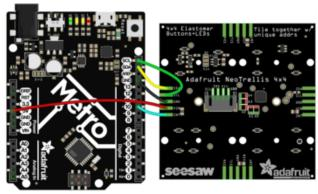
Use the same wiring from before, but this time connect **INT** to digital pin **#10** (you can change this later)
