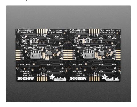
Perfect for your next cool interface, MIDI instrument, control panel...whatever could benefit from beautiful diffused colorful buttons. For fast connection to a single board, we include a JST-PH 4-pin connector that will give you power+data access. It's Grove compatible (the cable fits, even though its not the exact same connector), or you can use a JST-PH 4 pin cable (http://adafru.it/3568).
