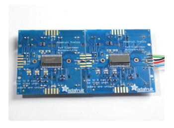
Solder two blobs of solder on two adjacent finger pads.
