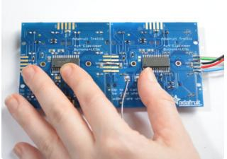
Use your soldering iron to drag solder from one pad to another, with a little effort they'll stick together and make a connection. You can add more solder to make the connection stronger. Its still not mechanically strong - so be careful not to bend or shake the arrangement
