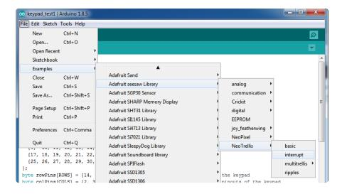
The behavior is identical to the **basic** example, but the INT pin is used instead of polling the NeoTrellis for new data. This frees up more time for your host microcontroller to do other things!
