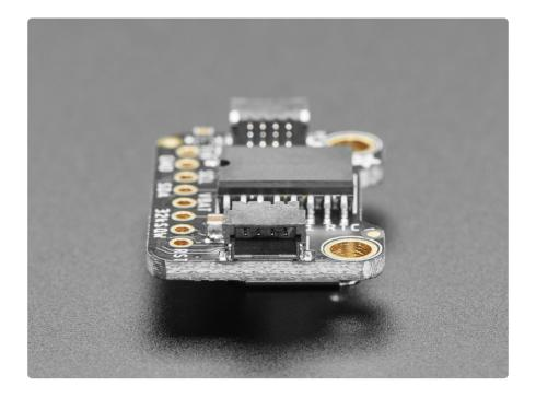
Comes as a fully assembled and tested breakout plus a small piece of header. You can solder header in to plug it into a breadboard, or solder wires directly.
