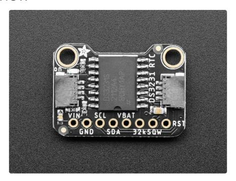
The datasheet for the DS3231 explains that this part is an "Extremely Accurate  $I^2C$ -Integrated RTC/TCXO/Crystal". And, hey, it does exactly what it says on the tin!  $\pm 2ppm$  accuracy from 0°C to  $\pm 40$ °C. This means  $\pm 1$  minute/year.
