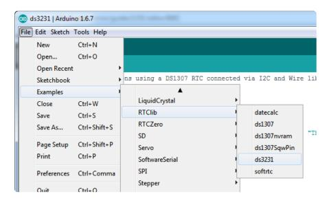
Upload to your Arduino and check the serial console @ 57600 baud (this is a change from the photos). After a few seconds, you'll see the report that the Arduino noticed this is the first time the DS3231 has been powered up, and will set the time based on the Arduino sketch.
