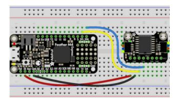
Vin (red wire) connected to your board's 3.3V or 5V output.
