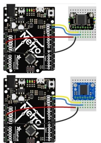
Connect Vin (red wire) to the power supply, 3-5V is fine. Use the same voltage that the microcontroller logic is based off of. For most Arduinos, that is 5V Connect GND (black wire) to common power/data ground
