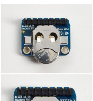
Don't forget that the Real Time Clock requires a battery backup. A CR1220 size battery goes in the back, make sure the + symbol on the battery is visible when you insert!
