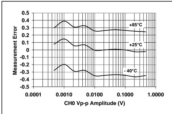
**FIGURE 2-8:** Measurement Error, Gain = 2, PF = 1.
