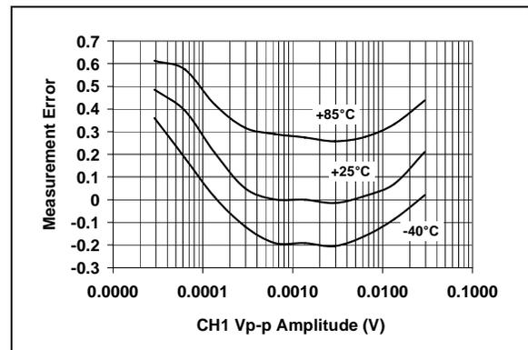
**FIGURE 2-5:** Measurement Error, Gain = 16, PF = 0.5.
