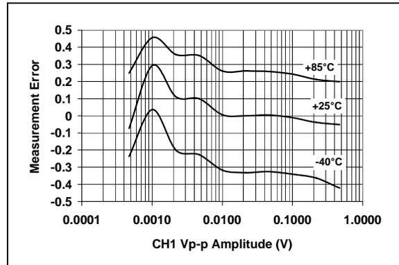
**FIGURE 2-10:** Measurement Error, Gain = 2, PF = + 0.5.
