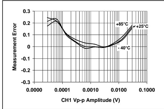
**FIGURE 2-19:** Measurement Error w/ External  $V_{REF}$  ( $G = 16$ ).
