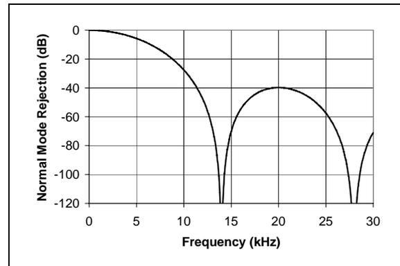
FIGURE 4-2: SINC Filter Magnitude Response ( $MCLK = 3.58$  MHz).
