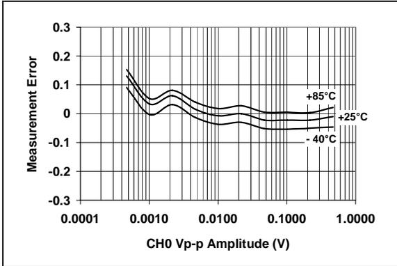
**FIGURE 2-17:** Measurement Error w/ External  $V_{REF}$  ( $G = 1$ ).
