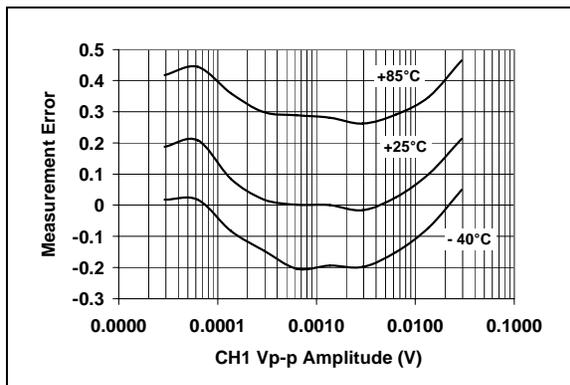
**FIGURE 2-2:** Measurement Error, Gain = 16, PF = 1.
