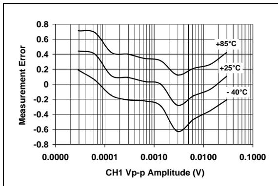
**FIGURE 2-3:** Measurement Error, Gain = 32, PF = 1.
