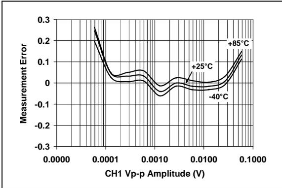
**FIGURE 2-18:** Measurement Error w/ External  $V_{REF}$  ( $G = 8$ ).
