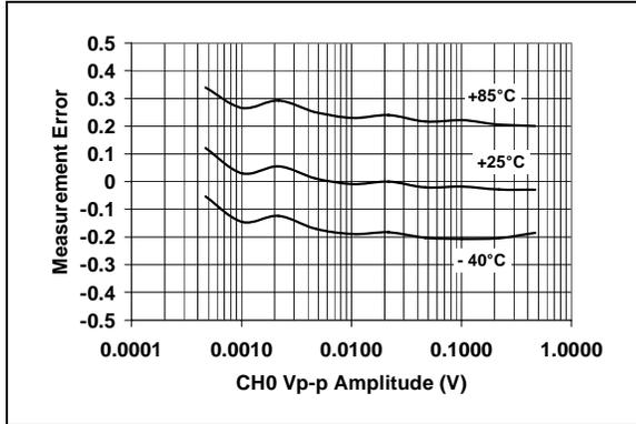
**FIGURE 2-7:** Measurement Error, Gain = 1, PF = 1.
