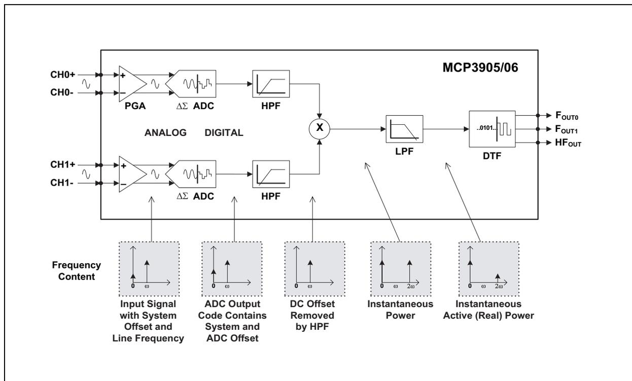
**FIGURE 4-1:** Simplified MCP3905/06 Block Diagram with Frequency Contents.
