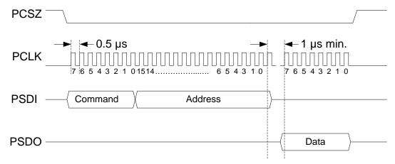
Figure 2: SPI Slave Port: Read Operation with Gap
