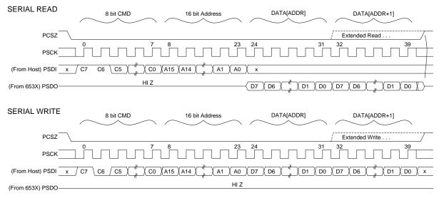
Figure 1: SPI Slave Port: Typical Read and Write operations
