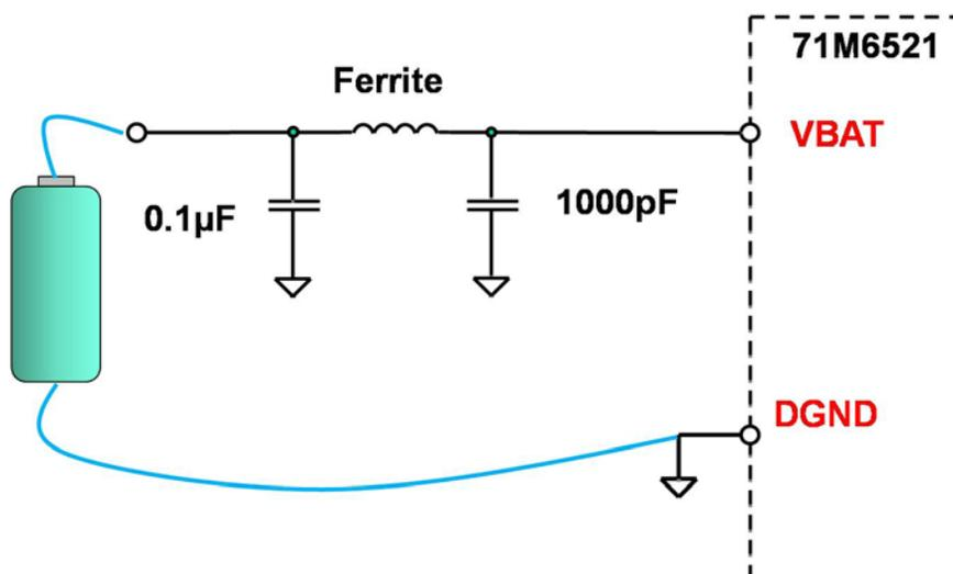
Figure 7: Components for the VBAT Pin
