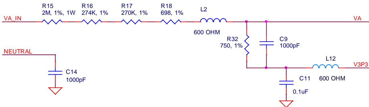
**Figure 11: Voltage Input Circuit for CT**
