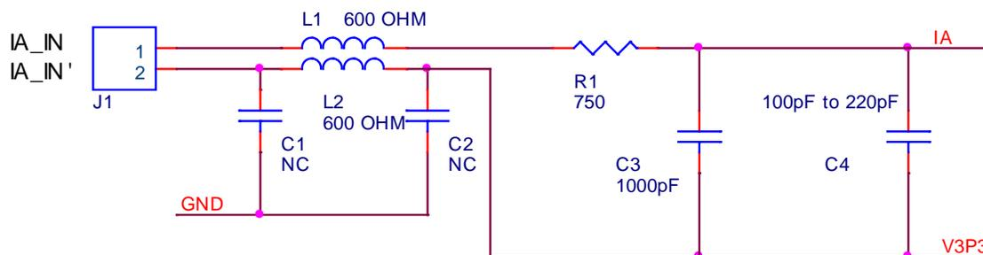
Figure 14: Current Shunt Input Signal Processing Circuit
