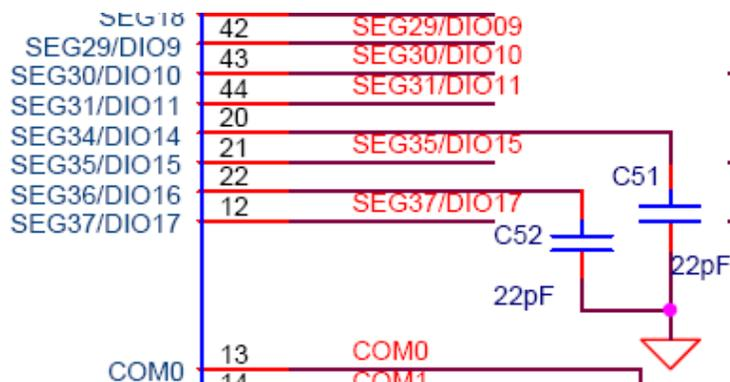
Figure 1: Termination for Unused LCD Pins
