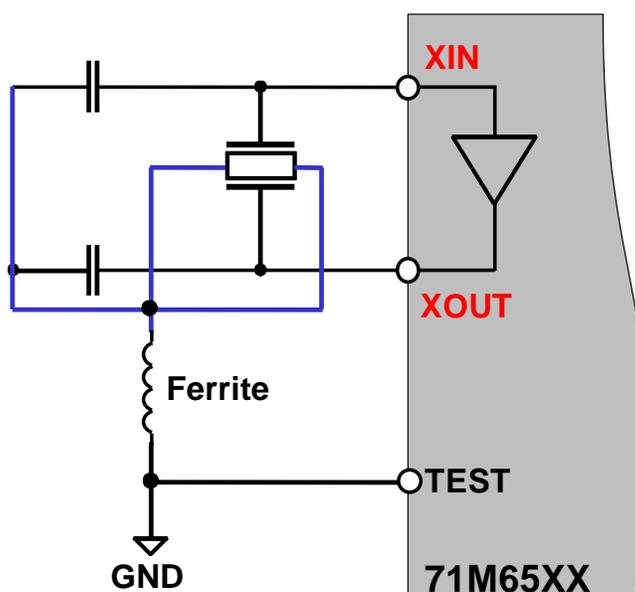
Figure 2: Connecting a Crystal to XIN/XOUT
