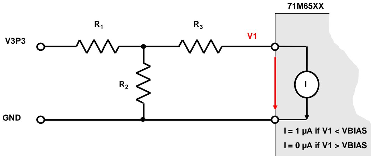
Figure 5: Generation of Hysteresis at the V1 Pin
