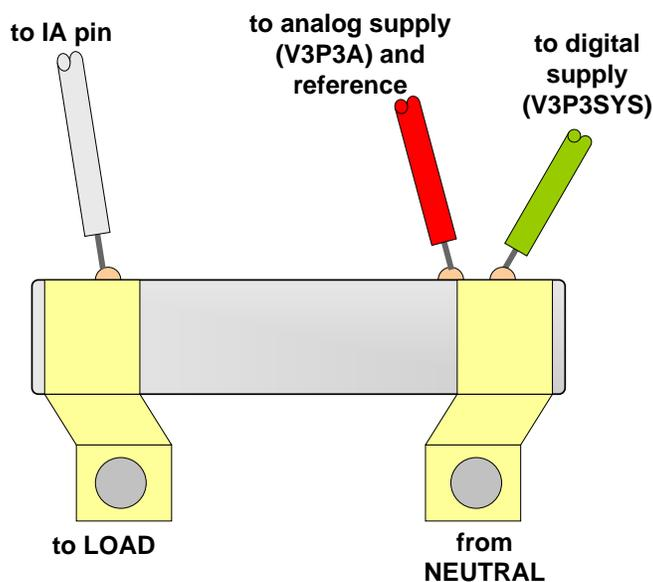
**Figure 12: Shunt Connections**
