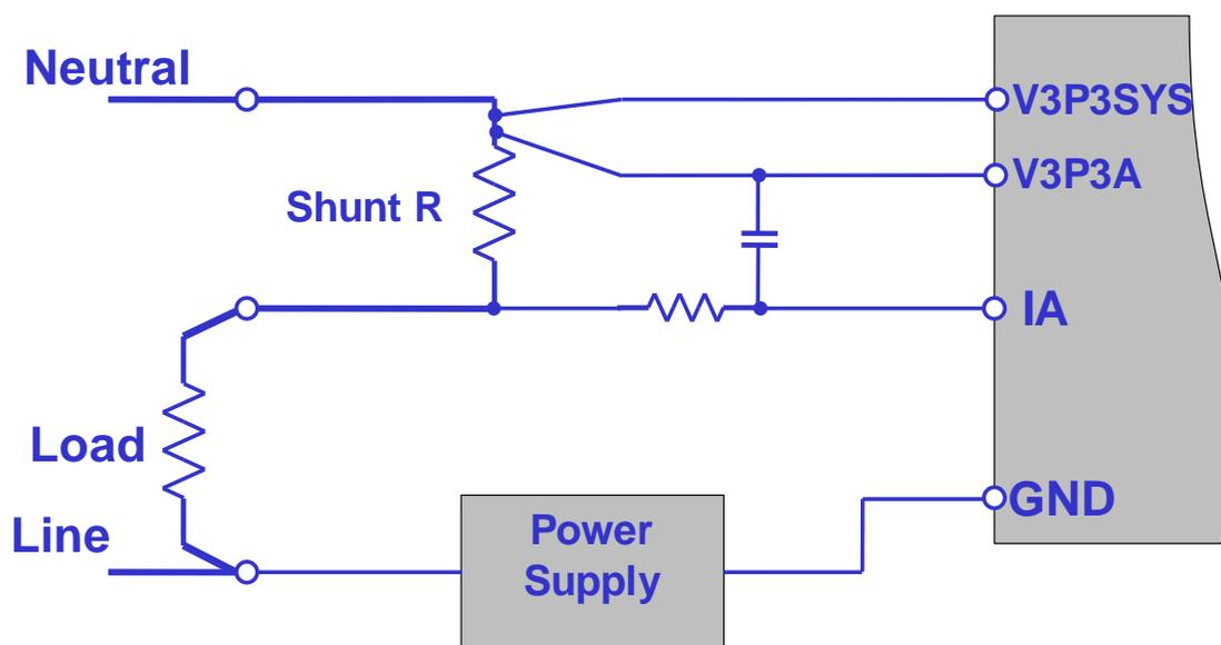
Figure 13: Current Shunt Circuit Topology
