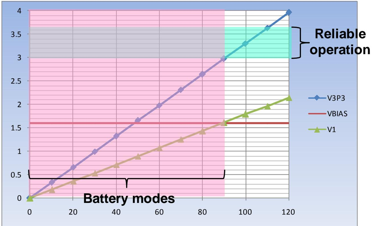
Figure 4: Operation Modes Controlled by the V1 Pin
