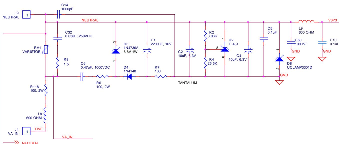
**Figure 15: Power Supply Circuit**
