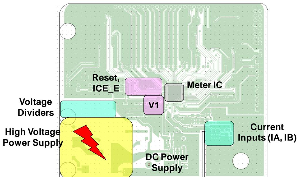
Figure 17: Component Placement
