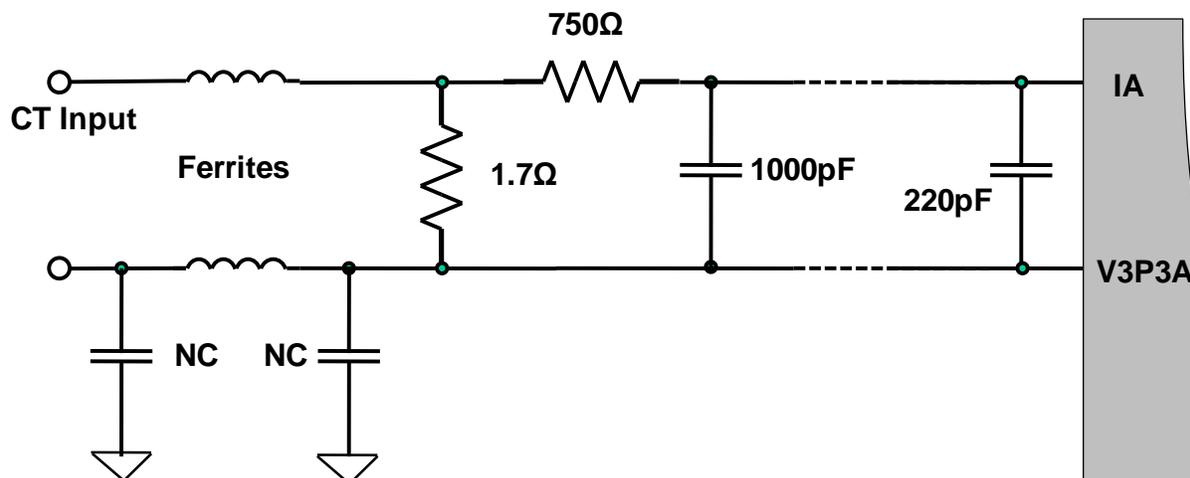
Figure 10: CT Input Signal Processing Circuit
