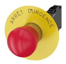
EMERGENCY STOP mushroom pushbutton, 22 mm, round, metal, shiny, red, 40 mm, positive latching, acc. to EN ISO 13850, pull-to-unlatch mechanism, with yellow backing plate, inscription: Arrêt d'urgence, with holder, 1 NO+1 NC, screw terminal, Z=20-unit packaging
