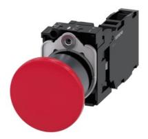
Mushroom pushbutton, 22 mm, round, plastic with metal front ring, red, 40mm, latching, pull-to-unlatch mechanism, with holder, 1 NO+1 NC, screw terminal, with laser labeling, symbol number according to, ISO 7000 or IEC 60417
