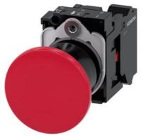
Mushroom pushbutton, 22 mm, round, plastic, red, 40mm, latching, pull-to-unlatch mechanism, with holder, 1 NC, spring-type terminal, with laser labeling, upper case and lower case, always upper case at the beginning of the word
