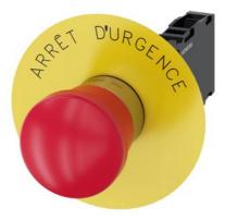
EMERGENCY STOP mushroom pushbutton, 22 mm, round, metal, shiny, red, 40 mm, positive latching, acc. to EN ISO 13850, pull-to-unlatch mechanism, with yellow backing plate, inscription: Arrêt d'urgence, with holder, 1 NO+1 NC, screw terminal
