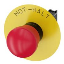
EMERGENCY STOP mushroom-type actuator, 22 mm, round, plastic, red, 40 mm, positive latching, according to EN ISO 13850, pull-to-unlatch mechanism, with yellow backing plate, inscription: NOT-HALT, with holder, 1 NC, screw terminal
