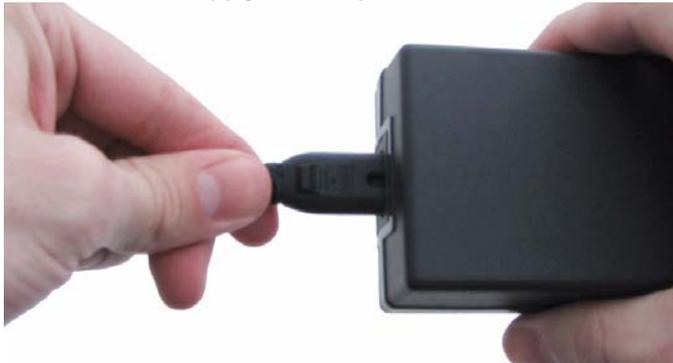
4. Plug the power adapter into an electrical outlet and the 5V line output connector into the power-in connector on the baseboard. See Figure 2.7.
