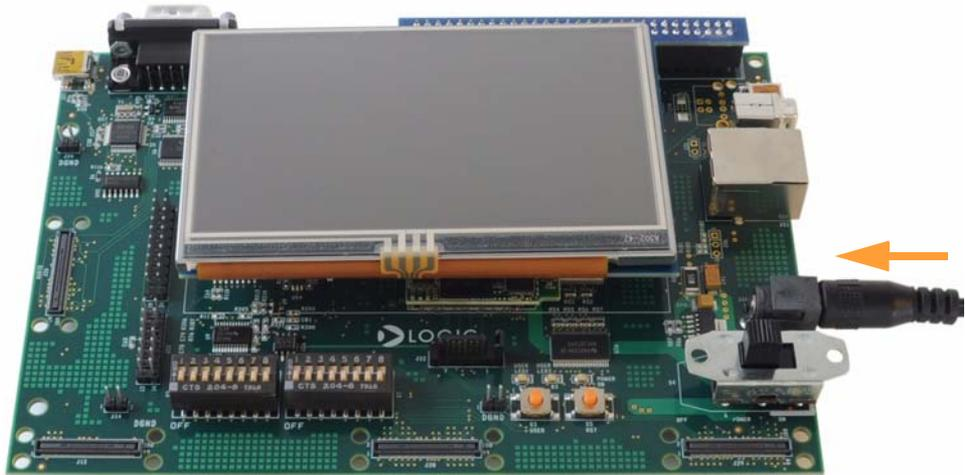
5. Verify the baseboard DIP switches are all set in the “OFF” position. Refer to Figure 1.2 for location of DIP switches on the baseboard.
