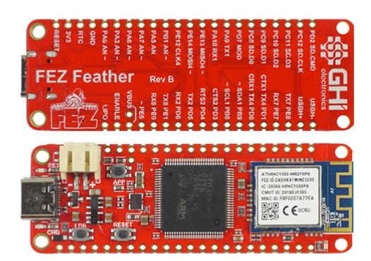
The Adafruit Feather form factor boards are made to be stackable and have built-in support for 3.7V LiPo batteries with a charging circuit. The **FEZ Feather** provides both through hole pads and castellated edges making it both breadboard friendly and easy to build into products.
