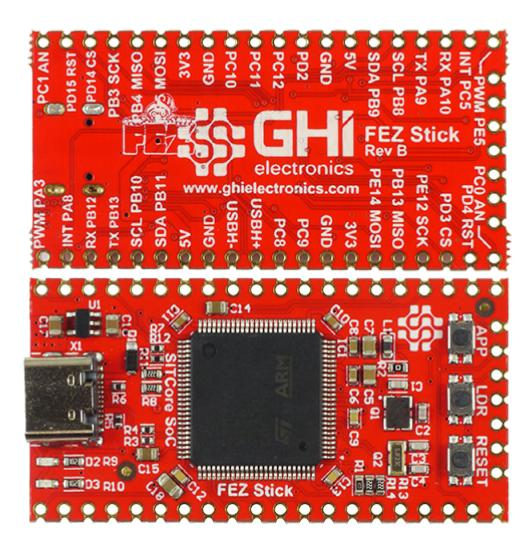
The **FEZ Stick** is a cost effective way to easily get started with TinyCLR OS. While providing an inexpensive way for the uninitiated to try TinyCLR OS, we've provided castellated edges as well as through hole pads to make it breadboard friendly and easy to embed into products. Also, there's actually space for two click modules, making this a very versatile board at a very affordable price!
