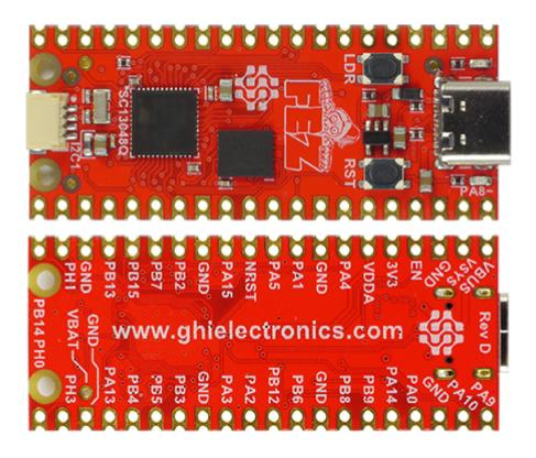
The **FEZ Pico** uses the Raspberry Pi Pico form factor allowing it drop into existing Pico accessories. The FEZ Pico adds JST connector compatible with Sparkfun Qwiic modules and Adafruit STEMMA modules. This allows for easy expandability.
