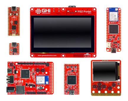
We offer multiple single board computers to provide the lowest possible barrier to entering the world of TinyCLR OS. Most of these boards have WiFi and they all support the complete TinyCLR feature set. These boards are great for trying out TinyCLR OS, building prototypes, or incorporating into products.
