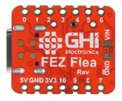
The **FEZ Flea** is the most cost effective way to dive into TinyCLR OS. With it's Seeeduino Xiao form factor it can be used with many existing accessories on the market. The board also has castellated and through-hole pins. Making it ideal for using as a SoM or on a breadboard.
