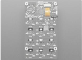
Above each set of key switch sockets, are RGB NeoPixel LEDs laid out in the same 3x4 grid. These reverse-mount LEDs are mounted to the back of the board to shine through to the front (to allow for the key switches to sit flush against the front of the board!).
