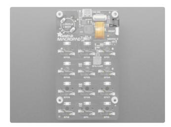
In the top right corner of the back of the board, below the mounting boss, is the STEMMA QT (https://adafru.it/Ft4) connector. This Qwiic-compatible I2C connector is designed to make it super simple to connect up STEMMA QT sensors and breakouts (https://adafru.it/Qgf).
