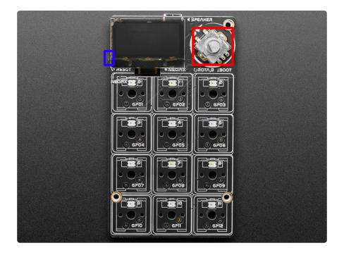
The BOOT button is the button switch in the rotary encoder! To engage the BOOT button, simply press down on the rotary encoder.
