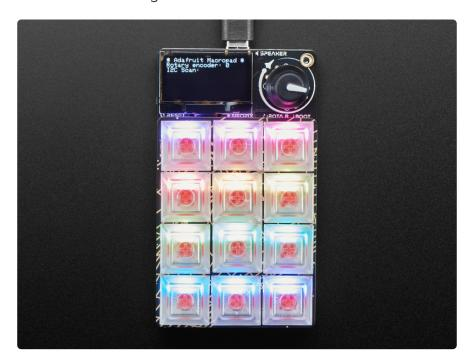
This space-ship is also fitted with a 128x64 monochome OLED for a crisp heads-up display that can be used in Arduino or CircuitPython to display keymaps, stats, computer performance, etc. There's also a rotary encoder with push-button soldered in. Twist and turn it or push to change volume or monitor brightness or scroll: whatever you like! A tiny speaker can give audio feedback or play fun bleepy tunes.
