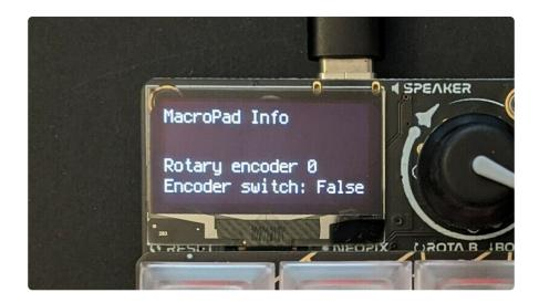
If you rotate the rotary encoder, the number will change. It doesn't matter where the rotary encoder is, it will begin at 0. The number provided is a relative position.
