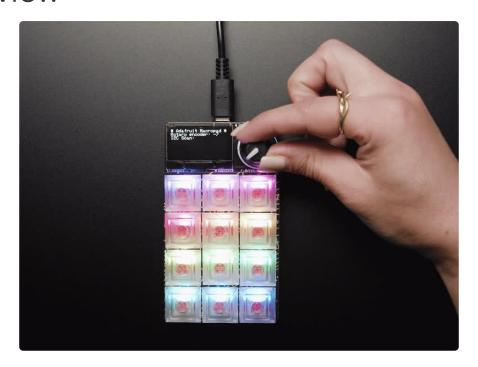
Strap yourself in, we're launching in T-minus 10 seconds...Destination? A new Class M planet called MACROPAD! M here, stands for Microcontroller because this 3x4 keyboard controller features the newest technology from the Raspberry Pi sector: say hello to the RP2040. It's speedy little microcontroller with lots of GPIO pins and a 64 times more RAM than the Apollo Guidance Computer. We added 8 MB of flash memory for plenty of storage.
