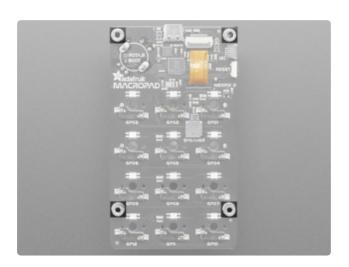
Arranged in the top two corners of the board, and towards the bottom two corners are four **mounting bosses** to allow for using the MacroPad enclosure kit (http://adafru.it/5103) or designing your own enclosures.
