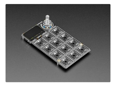
Get ready to upgrade your desk's mission control station with a CircuitPython or Arduino powered Macropad - complete with 12 buttons, OLED display, speaker and
