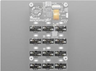
On the MacroPad, laid out in a 3x4 grid, are the **Cherry-MX compatible key switch sockets**. They are mounted on the back of the board so the socket points through to the front. The key switch sockets are individually tied to GPIO pins (i.e. not matrix-wired).
