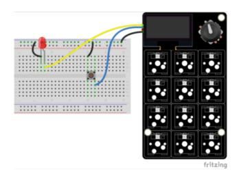
You can use either of the SCL and SDA pins from the STEMMA QT port as discreet GPIO, as long as they are not sharing a bus.
