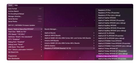
If there is no serial Port available in the dropdown, or an invalid one appears - don't worry about it! The RP2040 does not actually use a serial port to upload, so its OK if it does not appear if in manual bootload mode. You will see a serial port appear after uploading your first sketch.
