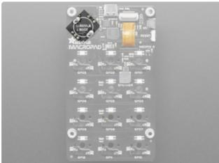
On the top right corner of the board (when viewed from the top), is the **rotary encoder** / **BOOT button**. The rotary encode has 20 detents per rotation. The BOOT button is required to enter the bootloader (needed for both CircuitPython and Arduino), and is also available as a user input in code. To use the button, simply press the rotary encoder down.
