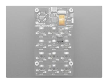
The grey square a bit to the right of the center of the board on the back is the **8mm speaker/buzzer**. With a Class D amplifier and RC filter, it can be used to make simple beeps and sounds effects.
