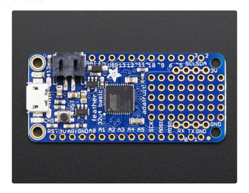
At the Feather 32u4's heart is at ATmega32u4 clocked at 8 MHz and at 3.3V logic, a chip setup we've had tons of experience with as <u>it's the same as the Flora</u> (http://adafru.it/659). This chip has 32K of flash and 2K of RAM, with built in USB so not only does it have a USB-to-Serial program & debug capability built in with no need for an FTDI-like chip, it can also act like a mouse, keyboard, USB MIDI device, etc.
