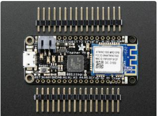
The first option is soldering in plain male headers, this lets you plug in the Feather into a solderless breadboard
