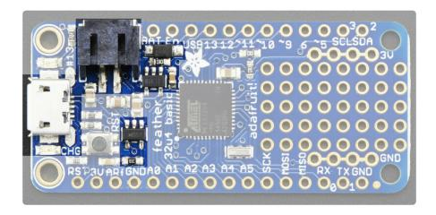
The above shows the Micro USB jack (left), LiPoly JST jack (top left), as well as the 3.3V regulator and changeover diode (just to the right of the JST jack) and the LiPoly charging circuitry (to the right of the Reset button).
