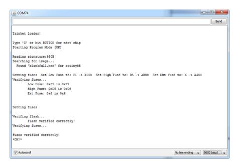
If you keep getting "Failed to verify fuses" while trying to restore the bootloader on a 3.3V Trinket using a Duemilanove. Try connecting 5V to the 3V pin on the Trinket, not VBAT+. Make sure USB is not plugged into the Trinket when you do this. Its a bit of a hack but may help!
