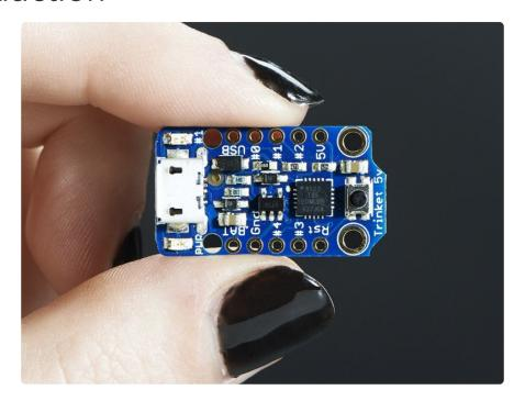
Trinket may be small, but do not be fooled by its size! It's a tiny microcontroller board, built around the Atmel ATtiny85, a little chip with a lot of power. We wanted to design a microcontroller board that was small enough to fit into any project, and low cost enough to use without hesitation. Perfect for when you don't want to give up your expensive dev-board and you aren't willing to take apart the project you worked so hard to design. It's our lowest-cost arduino-IDE programmable board!
