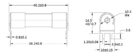
Note: recommended tightening torque is 4.5+/-1.0 Nm for M5 Screw
