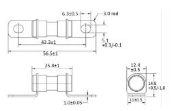
Note: recommended tightening torque is 4.5+/-1.0 Nm for M5 Screw
