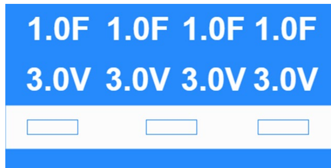
Example of the Markings of a 1.0F 3.0V capacitor
