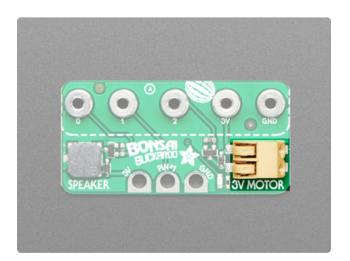
On the right is the **3V Motor control (on/off) on pin P2**. Connect to a water pump to automatically water dry plants. The **3V** connector (typically the red wire) goes into the part of the controller terminal towards the top, and the ground (typically the black wire) goes to the part of the controller terminal towards the bottom (by the **3V MOTOR label)**. However, for our pumps, it does not really matter which way you put the wires in
