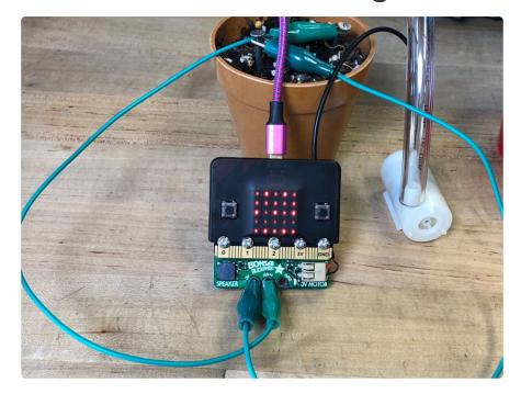
This example uses the Bonsai Buckaroo, the micro:bit, and Microsoft MakeCode to create an automatic plant care system.
