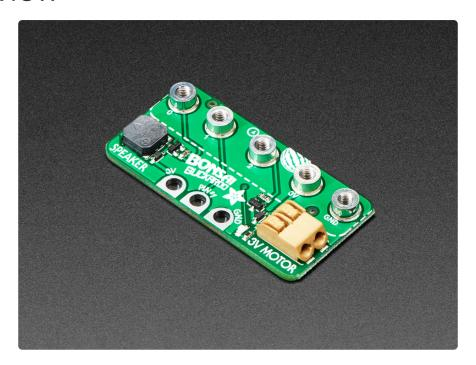
We can't wait for spring to arrive, and we're looking forward to caring for some plants! We designed this little add-on for <a href="micro:bit">micro:bit</a> (https://adafru.it/JFI) or <a href="CLUE">CLUE</a> (https://adafru.it/JFJ) boards – bolt it on with 5 screws to get a buzzer/beeper, motor driver, and breakouts for connecting a <a href="mailto:soil sensor">soil sensor</a> (https://adafru.it/JFK) (two alligator clips + nails work just fine). Simple, but effective!
