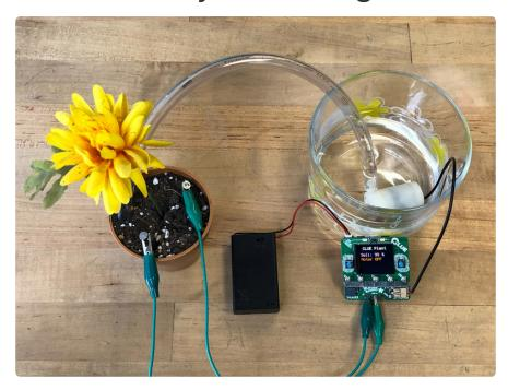
It's easy to use the Adafruit Bonsai Buckaroo with CircuitPython. This example uses the Adafruit CircuitPython CLUE (https://adafru.it/JFL) library to display soil moisture level and the status of the pump motor on the CLUE display. Connect your Bonsai Buckaroo to your CLUE, and connect the motor and plant to the Bonsai Buckaroo, and you're on your way to automatic plant care. Let's take a look!
