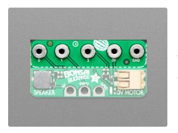
Along the top are the **mount points**. The Bonsai Buckaroo ships with screws for attaching to your micro:bit or CLUE.
