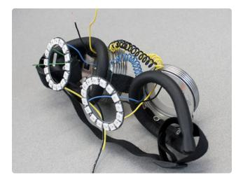
If using the "bring your own goggles" method, things may be a lot more complex...for example, these goggles have wires passing in and out through side perforations, so it's not possible to build and test the whole circuit separately first... it must be built around the goggles and is later folded into place. This is tricky!
