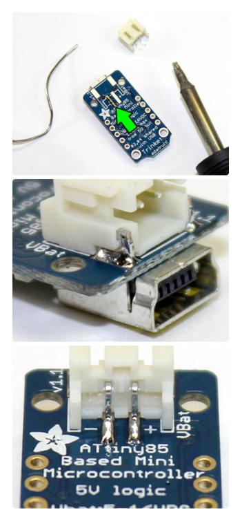
Start by "tinning" one of the JST pads on the back of the Trinket...heat the pad and apply solder so the whole surface is coated.
