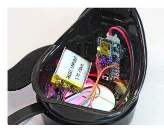
Power on the goggles by connecting the battery.
