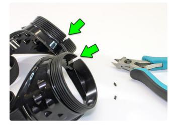
The costume goggles have slots near the nose piece, bridged by a tiny bit of plastic. If these are clipped away, then all the electronics can be slid in place from the front. You might also **cut the slots just a little wider** so they don't gouge the wires.
