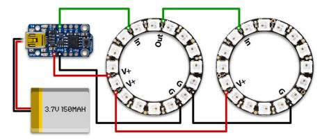
This diagram uses the original Trinket but you can also use the Trinket MO with the exact same wiring!
