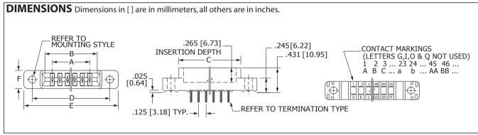
Tolerances on non-critical dimensions may very slightly due to shrinkage differential per insulator material; Consult factory.
