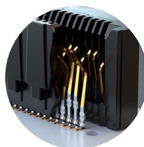
Differential pair for increased speed (HSEC8-DP)
