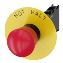
EMERGENCY STOP mushroom-type actuator, 22 mm, round, plastic, red, 40 mm, positive latching, according to EN ISO 13850, rotate-to-unlatch, with yellow backing plate, inscription: NOT-HALT, with holder, 1 NO+1 NC, spring-type terminal
