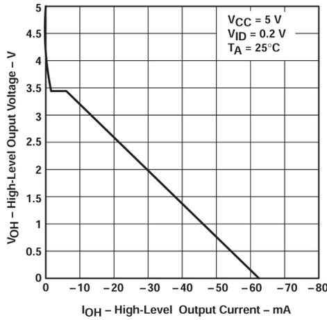
Figure 5-3. High-level Output Voltage vs High-level Output Current
