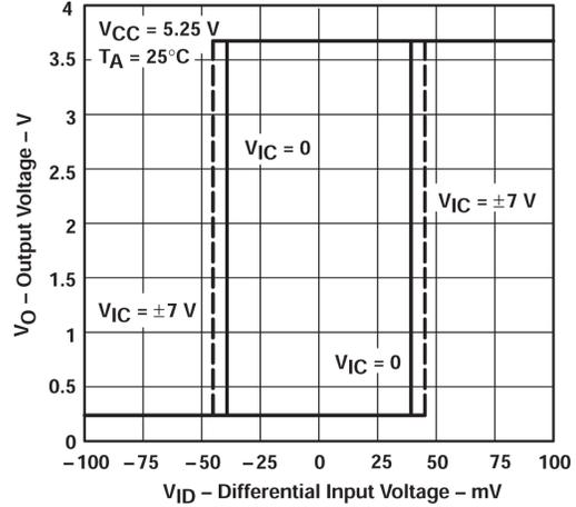
Figure 5-2. Output Voltage vs Differential Input Voltage
