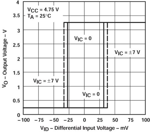
Figure 5-1. Output Voltage vs Differential Input Voltage
