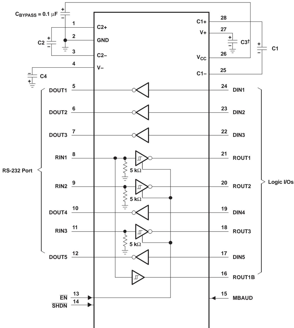
† C3 can be connected to V<sub>CC</sub> or GND.
