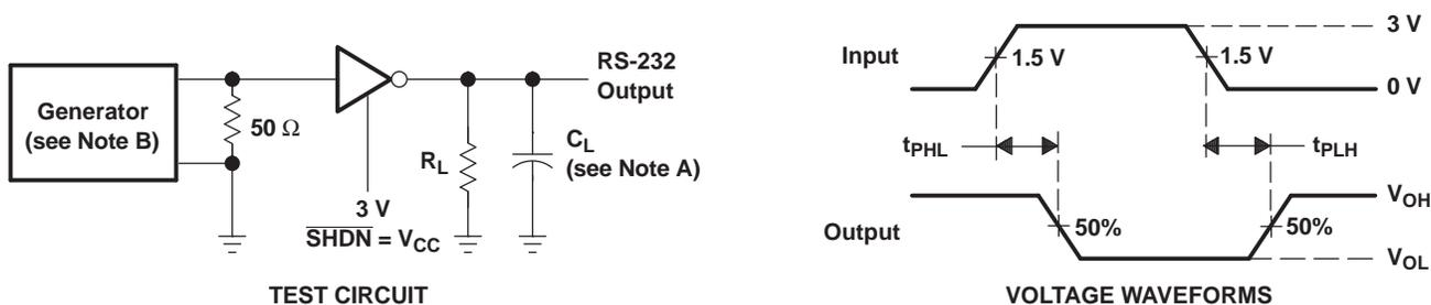
NOTES: A. C<sub>L</sub> includes probe and jig capacitance.
