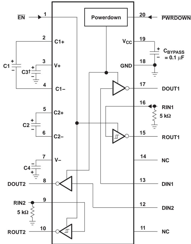
† C3 can be connected to  $V_{CC}$  or GND.
