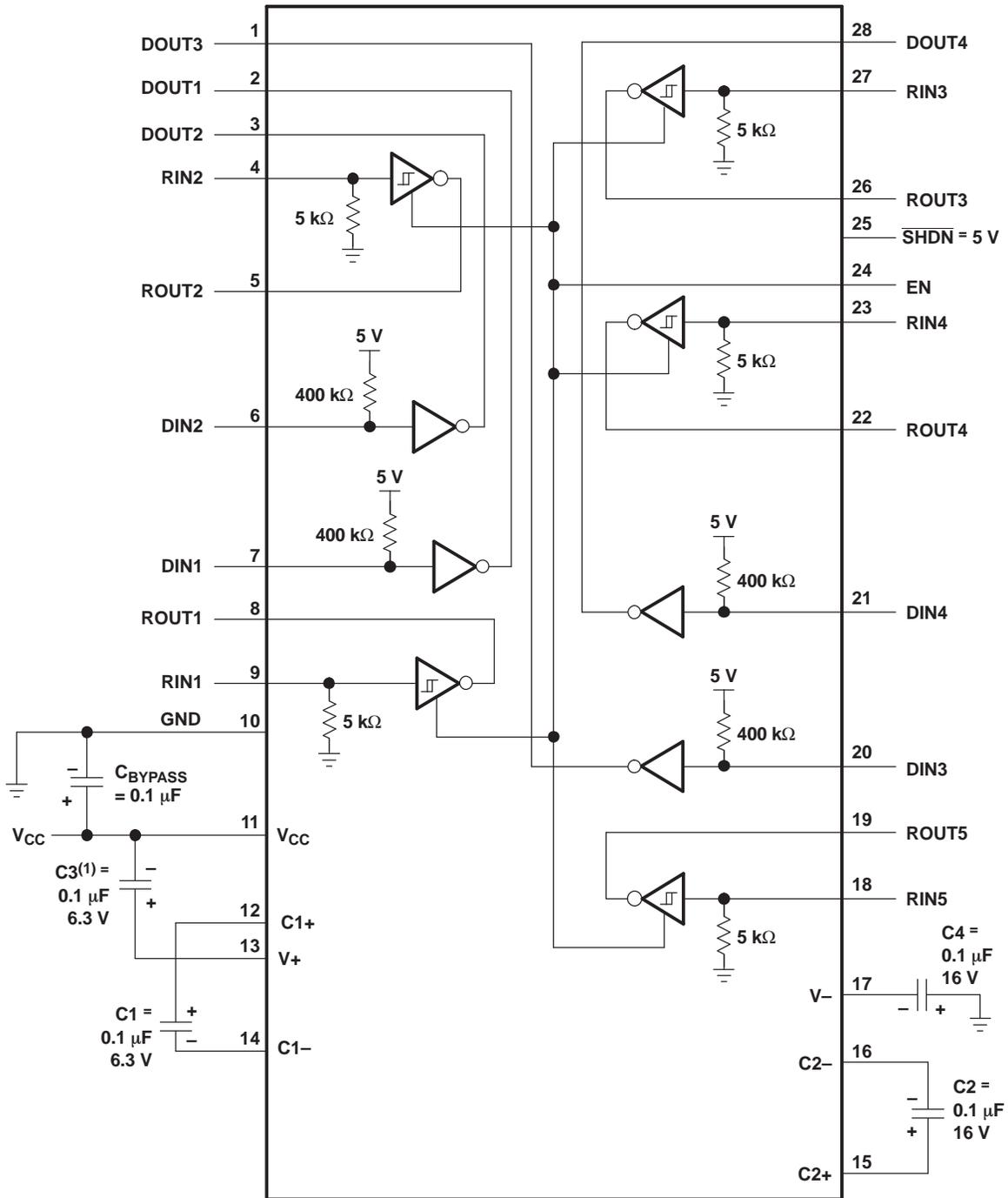
(1) C3 can be connected to  $V_{CC}$  or GND.
