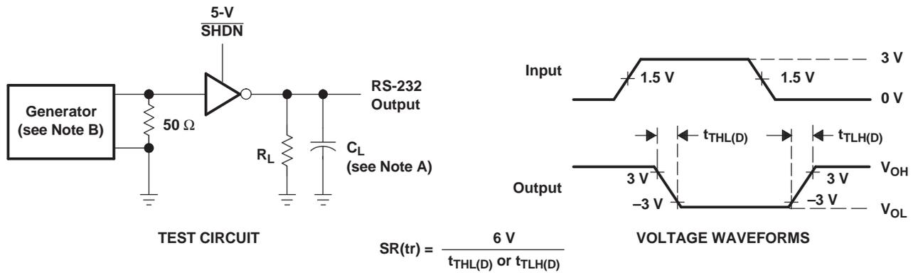
NOTES: A.  $C_L$  includes probe and jig capacitance.
